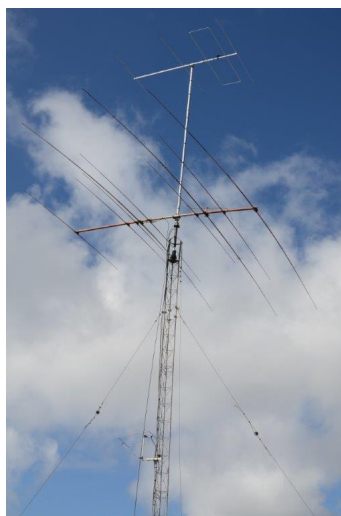
The 4 element 50MHz LFA-LN installed at ZD7VC
