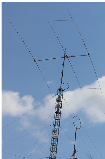
3el 20M OP-DES installed in 'JA'
