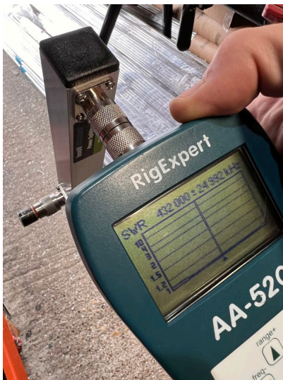
Analyser plot of a finished divider with sweep 25MHz either side of 432MHz
