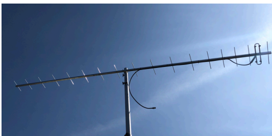
The 18e1 LFA-Ultra ready for connection to a masthead preamp
