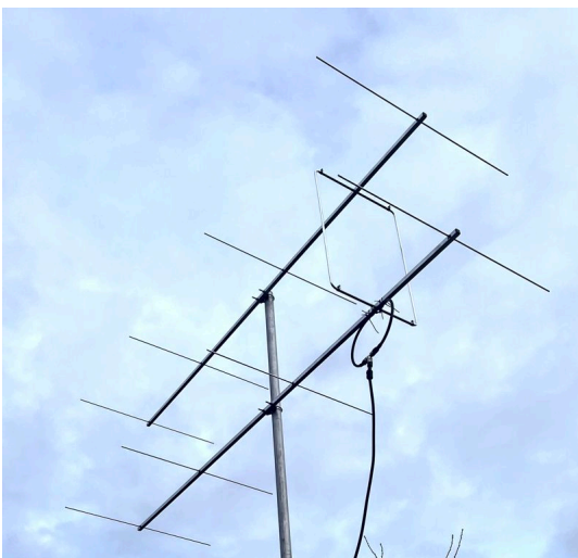
The 9el Slot-Q on test with the provided coaxial 'Loop' Balun. rear mounted version shown, centre mounted version also available.
