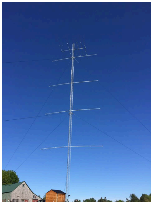
4 x 8el 11.7m 50MHz LFA-2 @ W2RE
