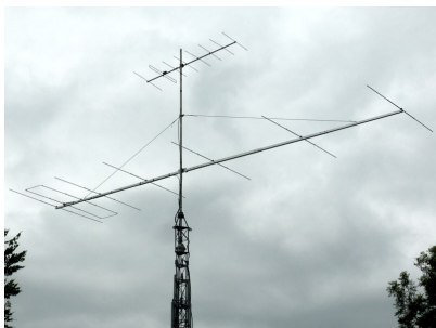
The 7el WOS installed are G2SJX
