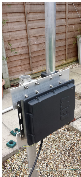
A typical installation with MFJ tuner installed with optional ATU mount fitted (VertiGo 43V pictured)
