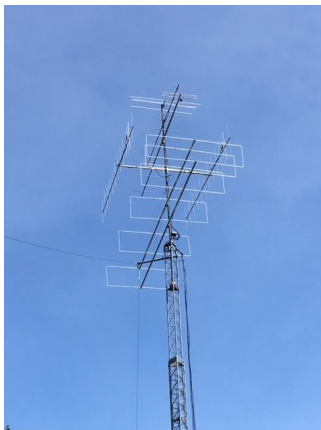
The 6el LFA-Q for 50MHz @ VE1PZ
