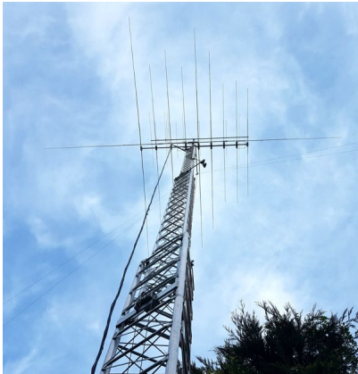
The 12el duo @ ON6ID above a 40m Rotating dipole and Optibeam HF Yagi
