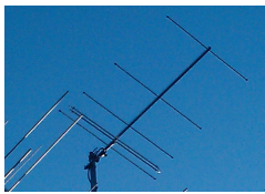
A 5 element OWL (Optimised Wideband Low Impedance) Super-Light Yagi for 144-146MHz
