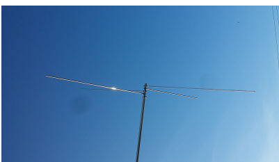
A close-up of the Capacity loaded end sections of the Delta C-140 and the 'spiral' configuration of the spokes
