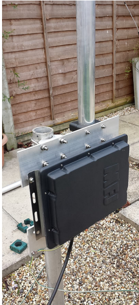
A typical installation with MFJ tuner installed (VertiGo 43V pictured). Optional ATU mount fitted
