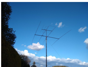
The 3el 17m low noise LFA Yagi @ Paul, M0AIA
