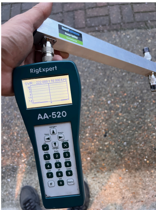
The 2 port 222MHz Power Divider has a flat response for around 11MHz either side of 222MHz
