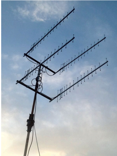
4 x 17el PMR-446 Yagis phased and stacked. For information on how to do this, contact us
