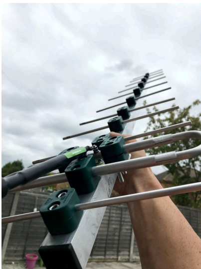
Looking down the barrel of the 11el 477MHz LFA Yagi
