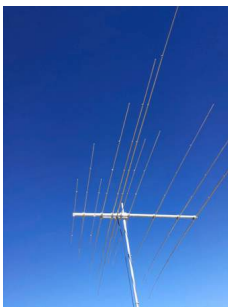
The XR6 MkII side view showing the short (3.5m) boom
