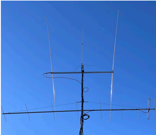
The BOLPA-2 on a tiny 2.1m boom installed and ready to go
