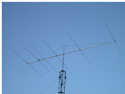
How the OP-DES looks; A 6el 28MHz OP-DES with single taper boom
