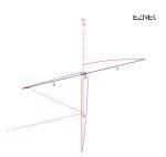
The above shows a Yagi fed with coax and no balun at the point at which the coax is connected. The current distribution is uneven through the driven element and the coax cable can be seen to be radiating too
