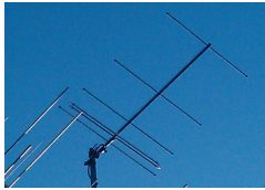
A 5 element OWL (Optimised Wideband Low Impedance) Super-Light Yagi for 144-146MHz
