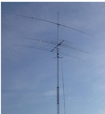
The Delta C-140 installed above an XR6 @ MONKR
