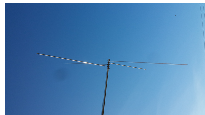
A close-up of the Capacity loaded end sections of the Delta 2-140 and the 'spiral' configuration of the spokes which are 8mm diameter
