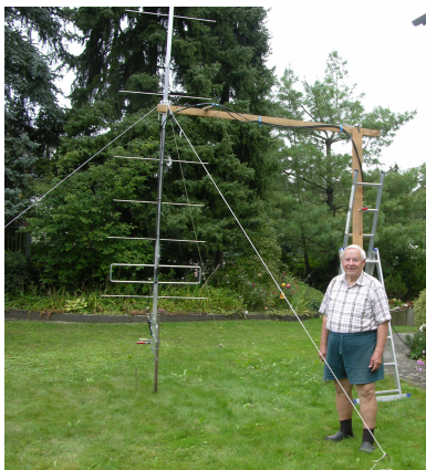
OE5KE stands beside one of his 20el LFA Ultra X-pols after testing SWR
