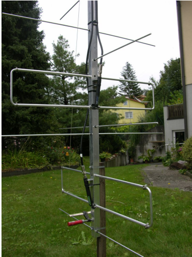
Close up of one of the 20el LFA Ultra X-pol Yagis @ OE5KE
