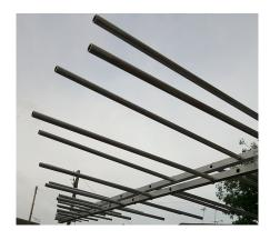
From under the antenna showing the full view including rear mounts and twin parasitic reflectors and directors
