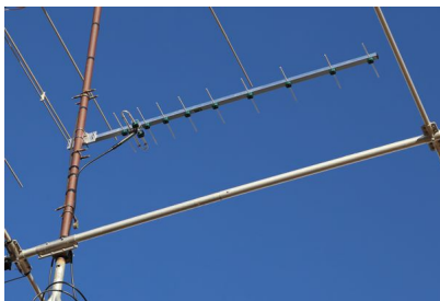
Rear mounted version of the 10el 430-435MHz LFA Yagi at Rob Sherwood, NC0B. Rob is the author of the Sherwood receiver Performance List.
