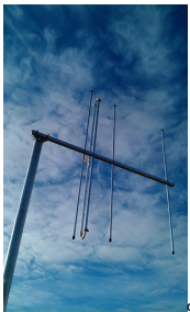
Custom Marine Band (155MHz - 157MHz) OWL Yagi -
