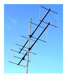
The 5el LFA-Q Long Boom installed at G0ElG
